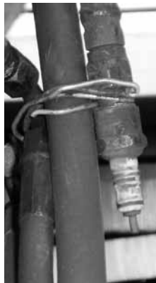
Needing to cap a hydraulic hose, Haitian mechanics used a spark plug because it was available.
