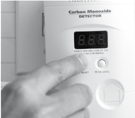
A carbon monoxide detector can save your life. Make sure to test the alarm according to the manufacturer's instructions. And replace the battery at least once a year.
